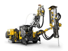
Bergteamet's Cable Bolt Rig for shafts has been developed for use in rock reinforcement with cable bolts in shafts.
